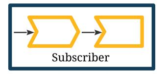
• Closed graphs. A closed graph has no inlet or outlet, both having being provided in during the construction of the graph. It is represented as a CompletionStage of the result of the stream. It contains a publisher stage, followed by zero or more processor stages, followed by a subscriber stage. This is called a CompletionRunner. The result is retrieved using the run method.
